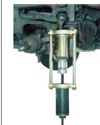
Press in lower ball joint
