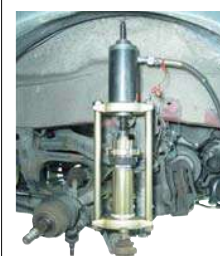
Press in upper ball joint
