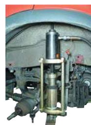
Press out upper ball joint
