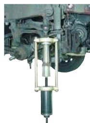
Press out lower ball joint
